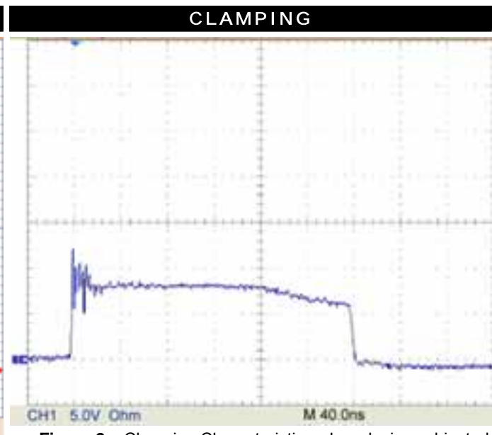
Figure 2 – Clamping Characteristics when device subjected to an 8 KV ESD pulse.
