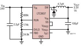
Figure 11. 24V to 3.3V, 1A Regulator at 200kHz
