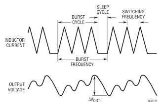
Figure 1. Burst Mode Operation
