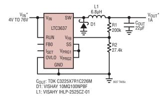
\*When V\_{IN} > 15V, LTC3637 SWITCHES AND V\_{0UT} IS REGULATED TO 15V; WHEN V\_{IN}  $\leq$  15V, LTC3637 OPERATES IN DROPOUT AND V\_{0UT} FOLLOWS V\_{IN}
