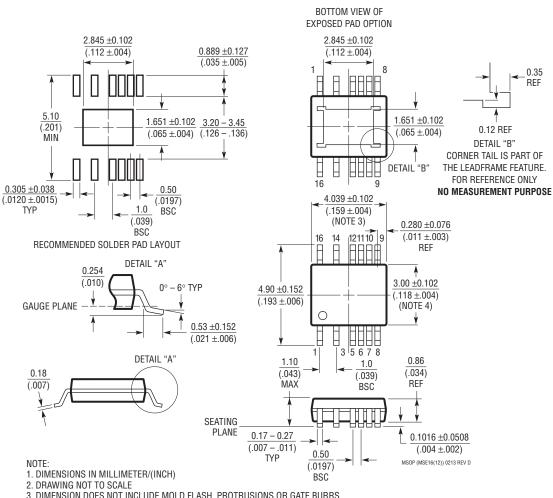
DIMENSION DOES NOT INCLUDE MOLD FLASH, PROTRUSIONS OR GATE BURRS. MOLD FLASH, PROTRUSIONS OR GATE BURRS SHALL NOT EXCEED 0.152mm (.006") PER SIDE
