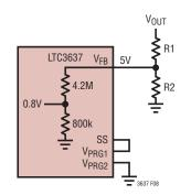
Figure 8. Setting the Output Voltage with External and Internal Resistors
