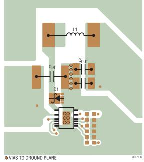
Figure 12. Example PCB Layout
