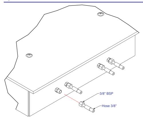
Take the minimum bend radius of the hoses into account when installing the hoses.
