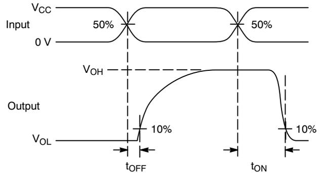
Figure 4.  $t_{ON}/t_{OFF}$
