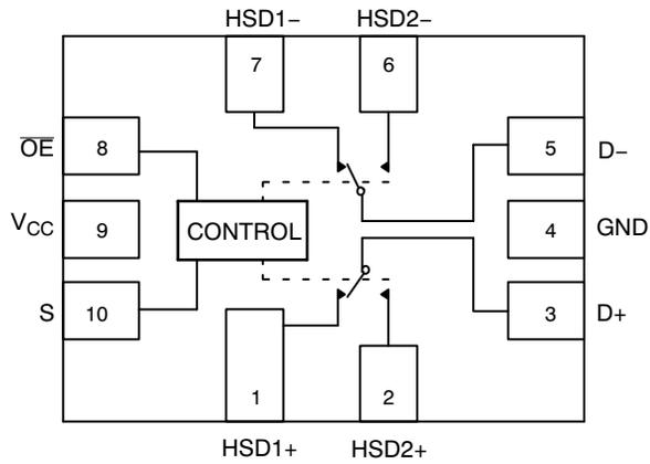
**Figure 1. Pin Connections and Logic Diagram**
