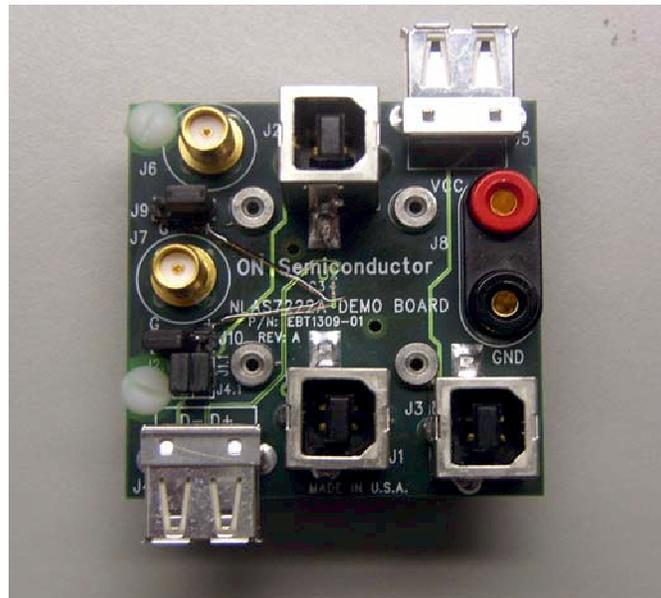
Figure 9. Photograph of the NLA57222A USB Demo Board
