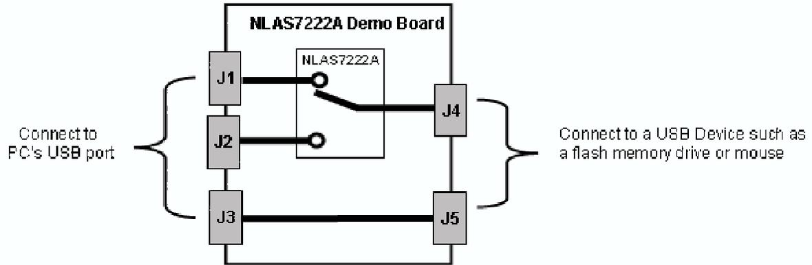
Figure 8. Block Diagram of the NLA57222A USB Demo Board
