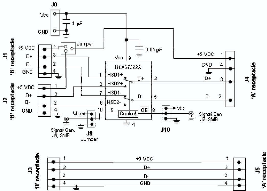
Figure 7. Schematic of the NLAS7222A USB Demo Board
