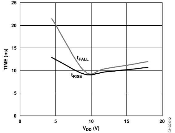
Figure 13. Rise and Fall Times vs.  $V_{DD}$
