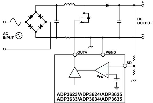
Figure 22. Shutdown Function Used for Redundant OVP
