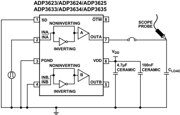
Figure 20. Test Circuit
