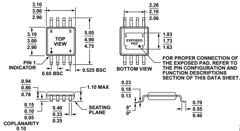
Figure 27. 8-Lead Mini Small Outline Package with Exposed Pad [MINI\_SO\_EP] (RH-8-1)
