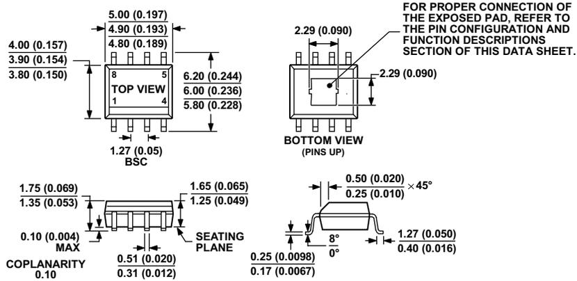
Figure 26. 8-Lead Standard Small Outline Package, with Exposed Pad [SOIC\_N\_EP] Narrow Body (RD-8-1)
