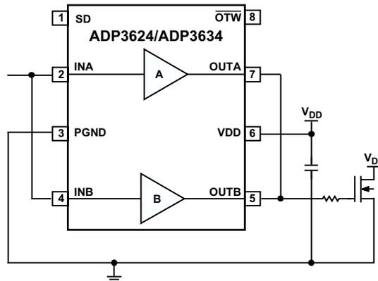
Figure 25. Parallel Operation
