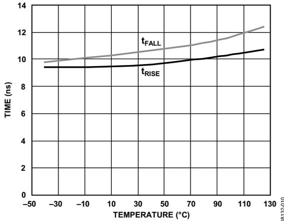
Figure 11. Rise and Fall Times vs. Temperature
