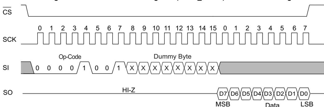
**Figure 8. Write Status Register (WRSR) Instruction Timing**
