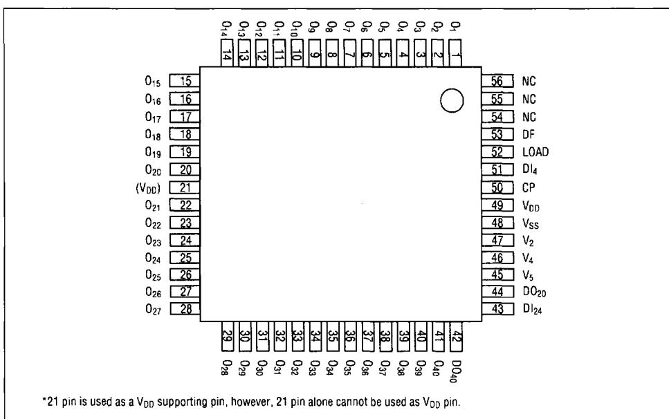
\*21 pin is used as a V<sub>DD</sub> supporting pin, however, 21 pin alone cannot be used as V<sub>DD</sub> pin.
