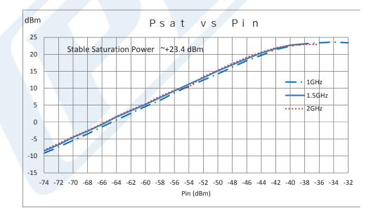
60 dB Gain, 19 dBm, 1 GHz to 2 GHz, Limiting Amplifer, -40 to 10 dBm Pin, SMA from Pasternack Enterprises has same day shipment for domestic and International orders. Our RF, microwave and millimeter wave products maintain a 99% availability and
