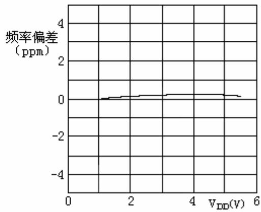
T<sub>A</sub>=25°C, normalized to V<sub>DD</sub>=3V
