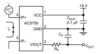
Application 1. The ACS750 outputs an analog signal, V<sub>OUT</sub>. that varies linearly with the uni- or bi-directional AC or DC primary sampled current, I<sub>P</sub>, within the range specified. C<sub>F</sub> is recommended for noise management, with values that depend on the application.
