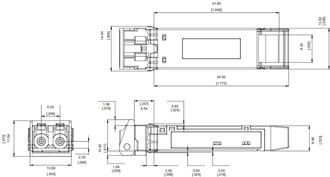
All dimensions shown are in [inches] and Millimeters. Millimeters are the primary units. Tolerances are in accordance with SFF-8432 Rev.5.
