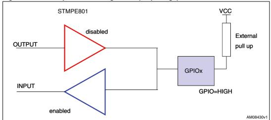
Figure 7. GPIO open drain configuration (output high)
