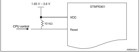
If reset delay and external reset assertion, as shown in case1 and case2 above, are not required, it is recommended to short the reset pin to VCC through a low resistor of 0.1 Ω - 100 Ω.
