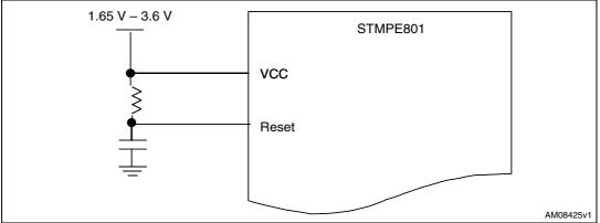
If external reset assertion is required through CPU/baseband, RSTB can be connected to the GPIO. The diagram below shows the presence of a weak pull-up resistor assuming CPU/baseband control is open drain. The minimum pulse width of the external reset signal is 100 µs.
