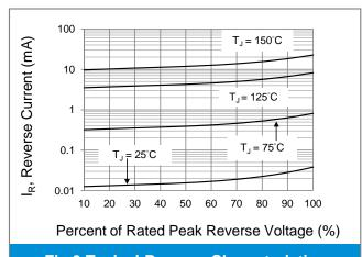
Fig.3 Typical Reverse Characteristics
