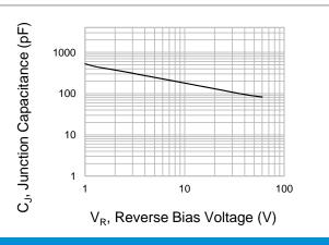
**Fig.2 Typical Junction Capacitance**
