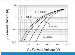
**Fig.4 Typical Forward Characteristics**
