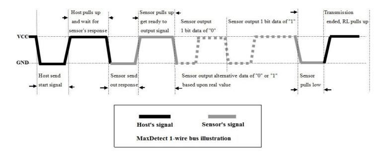
1) Step 1: MCU send out start signal to RHT01 and RHT01 send response signal to MCU
