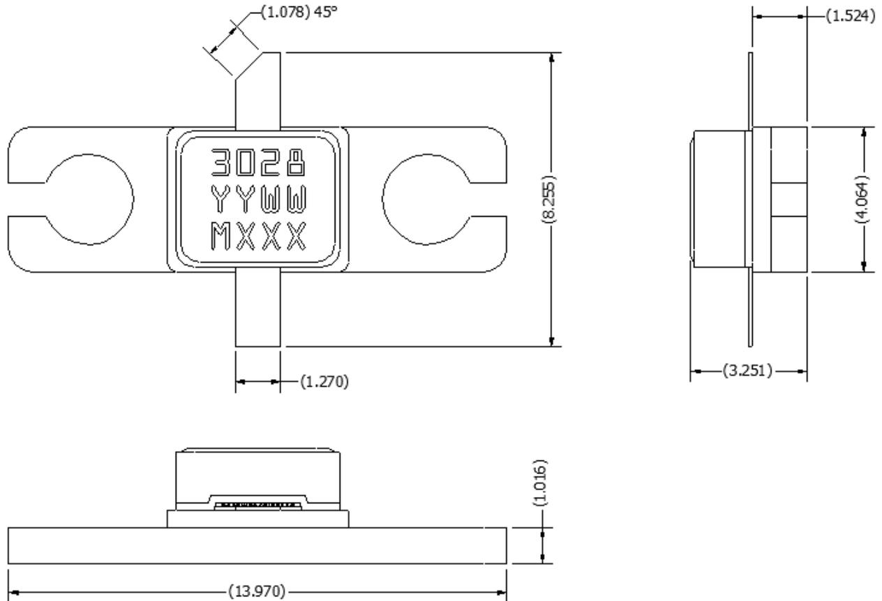
This package is lead-free/RoHS-compliant. The plating material on the leads is NiAu. It is compatible with both lead-free (maximum 260 °C reflow temperature) and tin-lead (maximum 245 °C reflow temperature) soldering processes.
