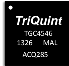
28-pin 5x5mm QFN package
