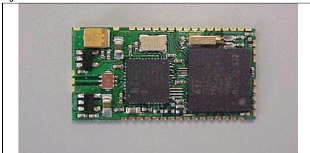
Figure 10. Bluetooth® wireless module BT-STA2416C2
