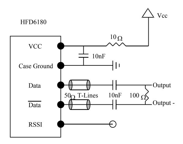
The  $100\Omega$  resistor prior to the limiting amplifier is needed only when the input impedance of the amplifier is not  $50\Omega$ DC blocking capacitors must also be present at the TIA outputs to avoid a large DC current which may damage the chip.
