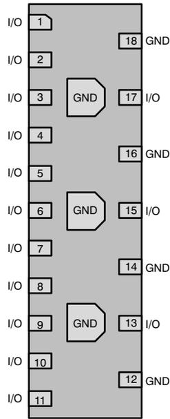
**Figure 2. Pin Configuration**
