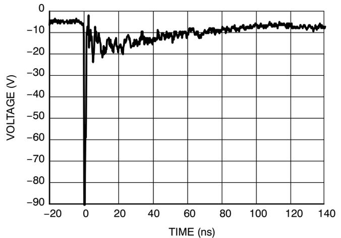
**Figure 4. IEC61000-4-2 -8 kV Contact Clamping Voltage**
