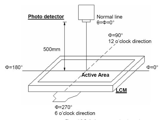
Figure 4.2 Optical measurement system setup
