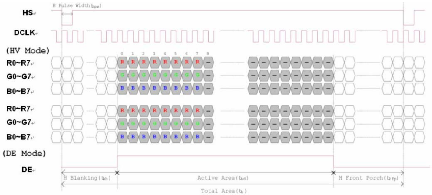
Figure 3.1 Horizontal input timing diagram.
