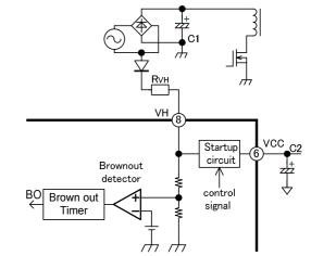
Fig. 19 Brown in and brown out detection circuit
