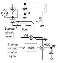
Fig.1 Startup circuit 1 (Half-wave)
