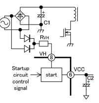
Fig.2 Startup circuit 2 (Full-wave)
