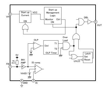
Fig.14 Overload protection circuit (timer latch)
