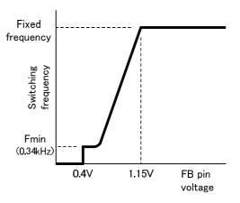
Fig.4 Oscillation frequency
