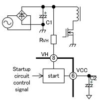
Fig.3 Startup circuit 3 (Rectification)
