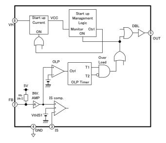
Fig.11 Overload protection circuit (auto recovery)
