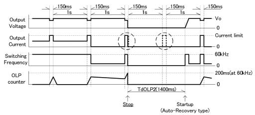
Fig. 13 Typical overload/light load repetition timing chart
