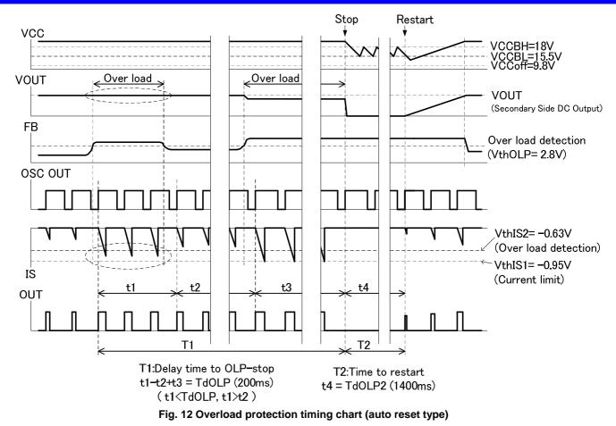
Since the OLP timer for overload protection delay time uses an up/down counter, a period for counting down is required to clear the count. Note that switching frequency (Fosc) is counted to detect the overload protection delay time (TdOLP).
