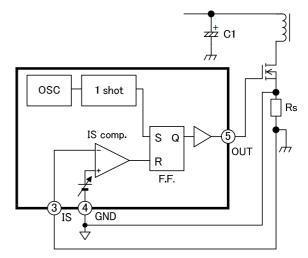
Fig.5 Current mode basic operation circuit block
