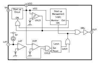
Fig. 18 Overvoltage protection circuit
