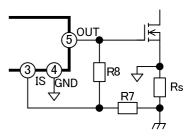
Fig. 32 Correction circuit for improvement of input power under light load
