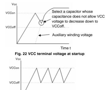
Time t Fig. 23 VCC terminal voltage at startup (when capacitance is too small)
