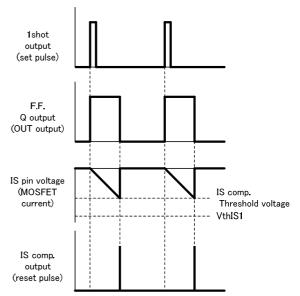
Fig.6 Current mode basic operation timing chart
