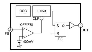
Fig.9 Output shutdown function of FB pin
