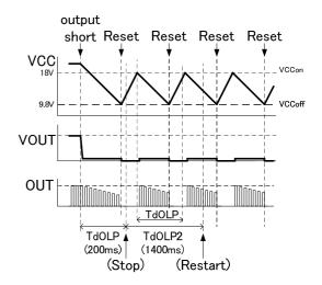
Fig. 25 VCC hold time (at output short circuit)
