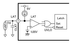
Fig. 17 Overheat protection function using a thermistor
