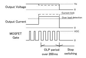
Fig. 10 Conceptual diagram of overload protection operation
