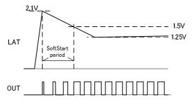
Fig. 16 LAT terminal soft start operation
