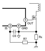
Fig. 30 IS terminal filter
