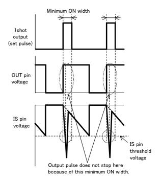
Fig.8 Minimum ON width
