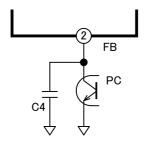
Fig. 29 FB terminal circuit configuration
