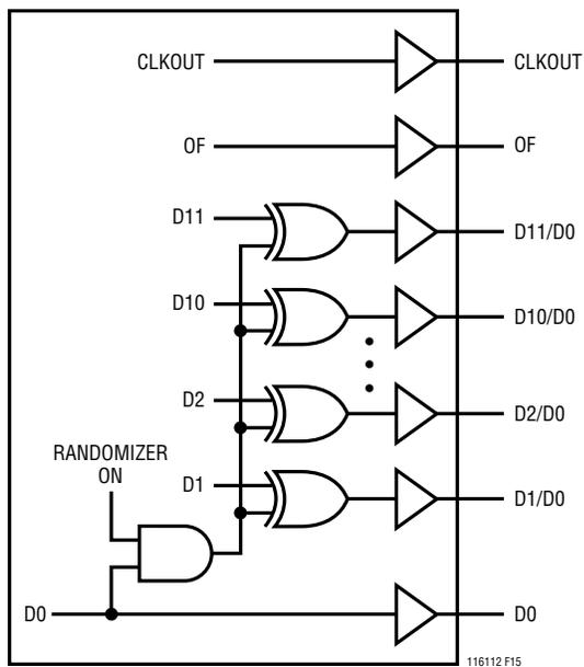
Figure 15. Functional Equivalent of Digital Output Randomizer
