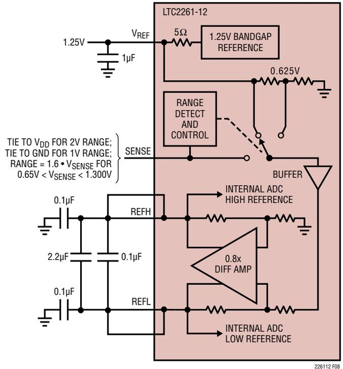
Figure 8. Reference Circuit
