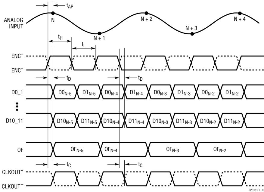
**Double-Data Rate LVDS Output Mode Timing**
