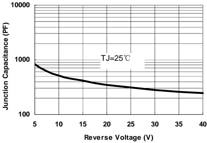
Fig.1-Typical Junction Capacitance
