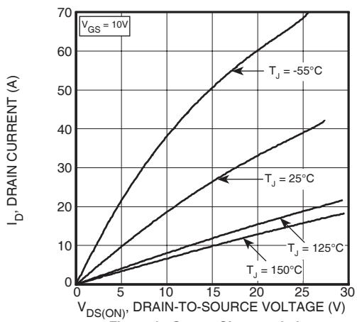
Figure 1, Output Characteristics
