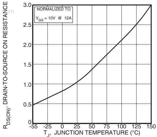
Figure 3,  $R_{DS(ON)}$  vs Junction Temperature
