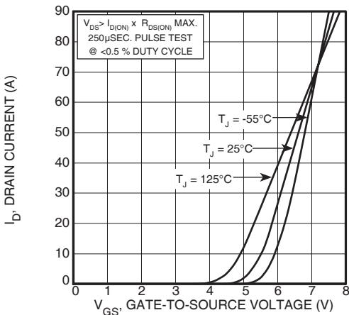
Figure 4, Transfer Characteristics
