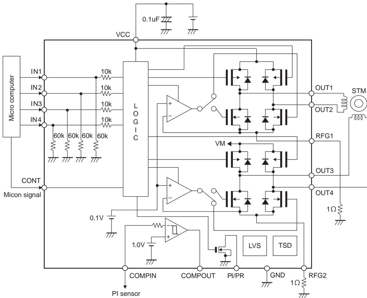
Constant-current calculation :  $I_{OUT} = 0.1 \div R_F$  Example : When an  $I_{OUT}$  of 100mA is required,  $R_F$  must be  $1\Omega$ .
