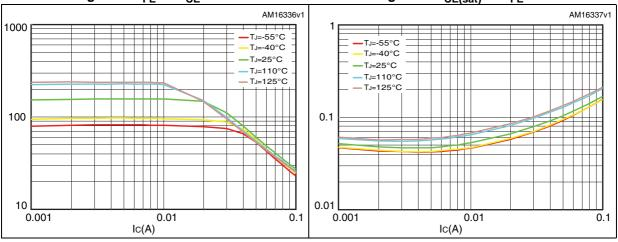
Figure 4. V<sub>BE(sat)</sub> @ h<sub>FE</sub> =10
