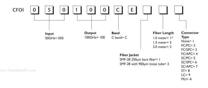
\* The tolerance of fiber length is +/-0.1 m. I meter is standard. The lead-time for special fiber length will be longer.
