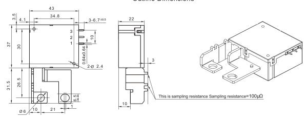
NOTE: The dimension of the load terminals as well as the sampling resistance can be made per customer request.
