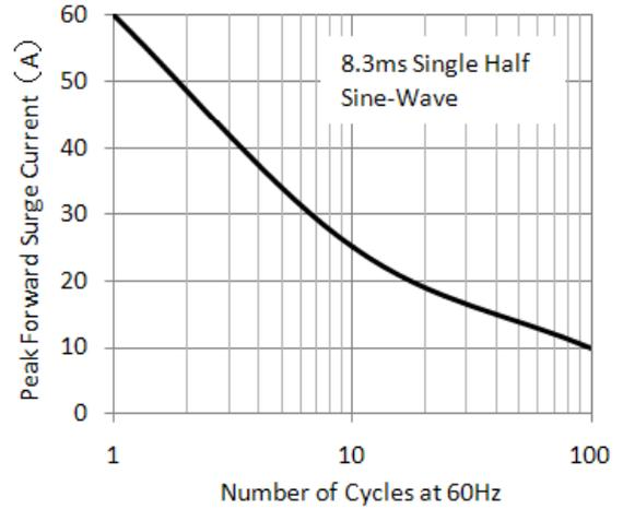
Figure 2. Maximum Non-Repetitive Peak Forward Surge Current
