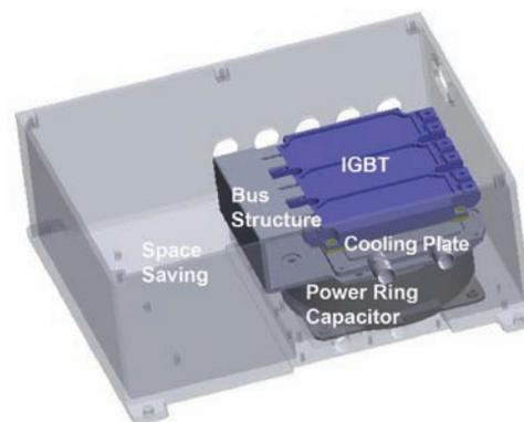
Figure 2 shows the “stacked” inverter design after the integration of the ring capacitor and the laminar bus plate. By now combining both aspects of vertical integration and the low temperature rise characteristics of the capacitors, an increase to 50% or more volume reduction is realistically possible. These improvements clearly translate into weight and cost reductions.
