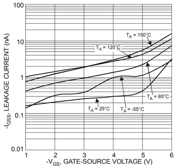
Figure 10 Typical Gate-Source Leakage Current vs. Voltage
