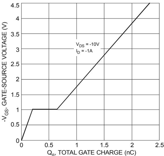
Figure 11 Gate-Charge Characteristics
