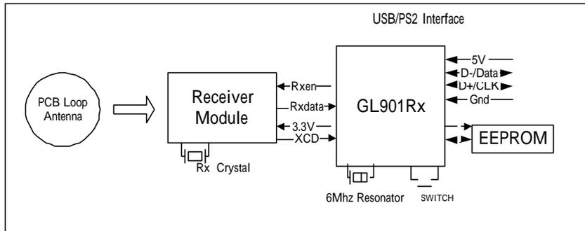
Figure 3-1: Block Diagram of RF Receiver System
