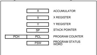
Figure 8-1 Configuration of Registers
