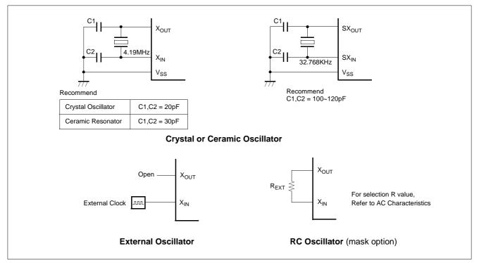
Figure 18-1 Oscillation Circuit
