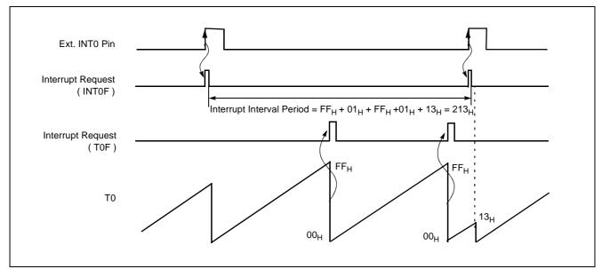
Figure 12-10 Excess Timer Overflow in Capture Mode
