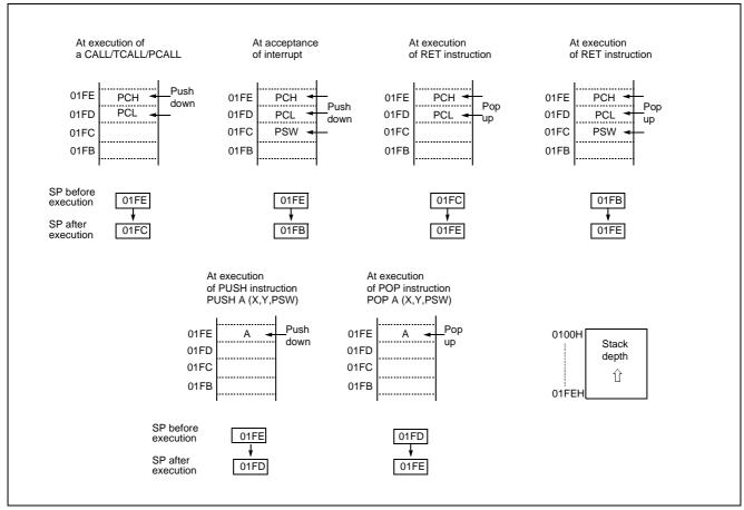
Figure 8-4 Stack Operation
