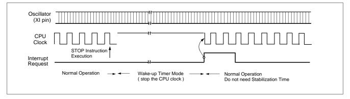
Figure 17-4 Wake-up Timer Mode Releasing by External Interrupt or Timer0 Interrupt
