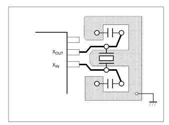
Figure 18-2 Layout of Oscillator PCB circuit
