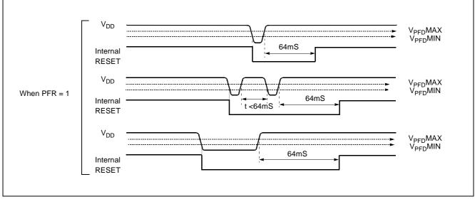
Figure 20-3 Power Fail Processor Situations
