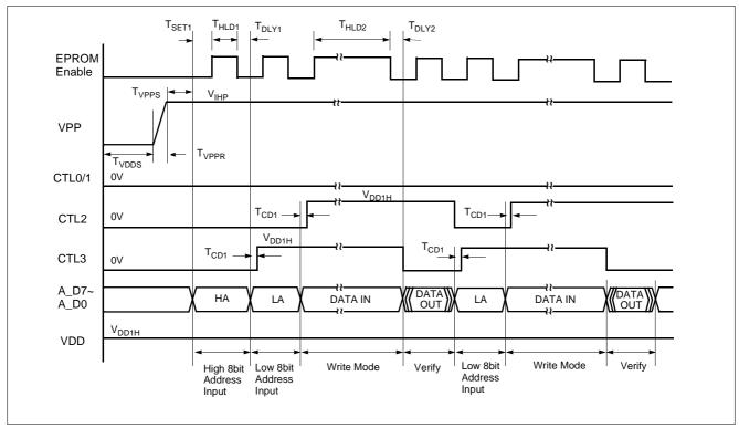
Figure 21-3 Timing Diagram in Program (Write & Verify) Mode
