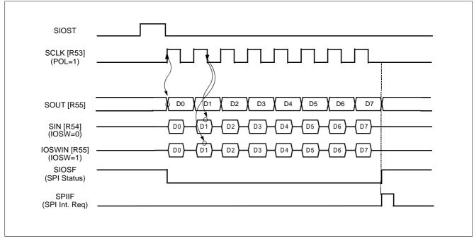
Figure 14-4 SPI Timing Diagram at POL=1
