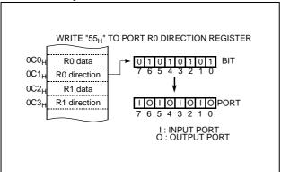
Figure 9-1 Example of Port I/O Assignment
