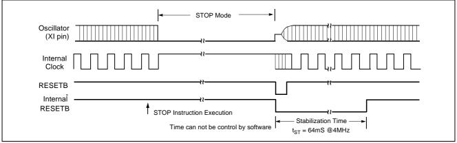
Figure 17-3 Timing of STOP Mode Release by RESET
