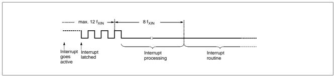
**Figure 16-8 Interrupt Response Timing Diagram**
