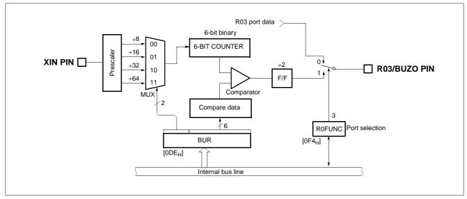
Figure 15-1 Block Diagram of Buzzer Driver
