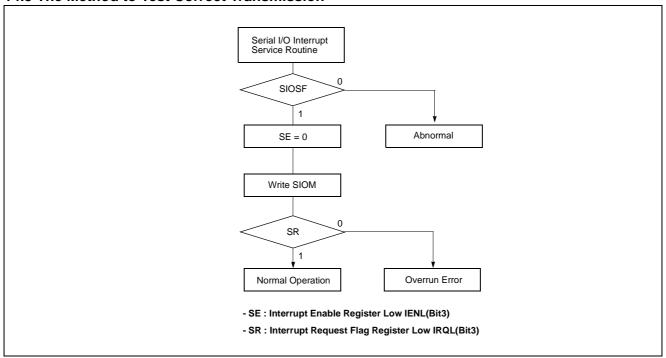
Figure 14-5 Serial Method to Test Transmission
