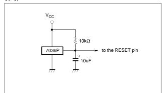
Figure 19-1 Simple Power-on-Reset Circuit
