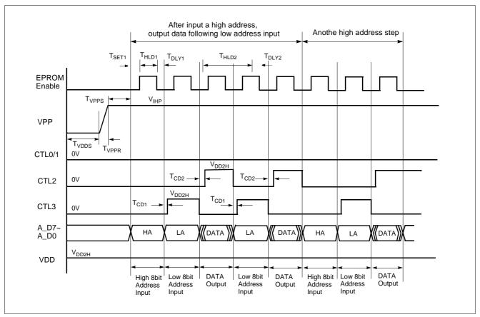
Figure 21-4 Timing Diagram in READ Mode
