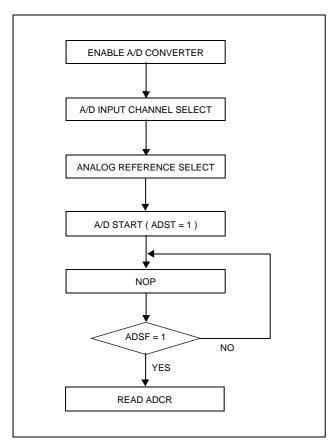
Figure 13-3 A/D Converter Operation Flow
