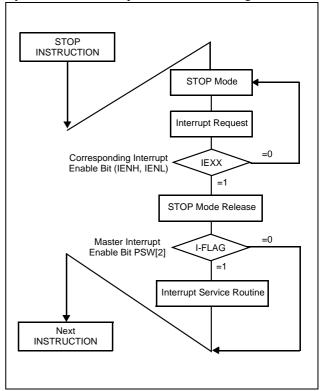
Figure 17-1 STOP Releasing Flow by Interrupts
