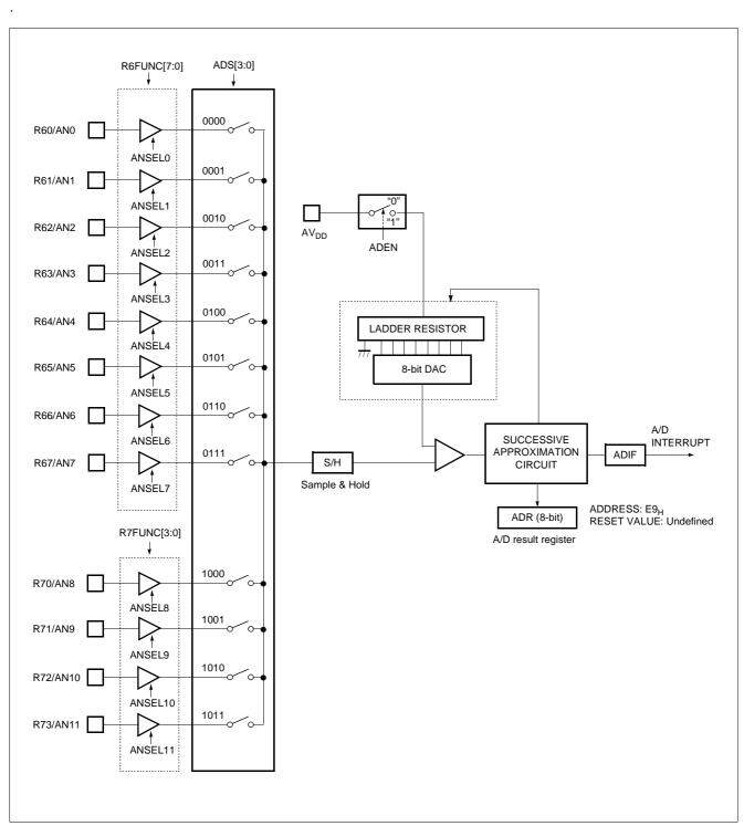
Figure 13-2 A/D Block Diagram
