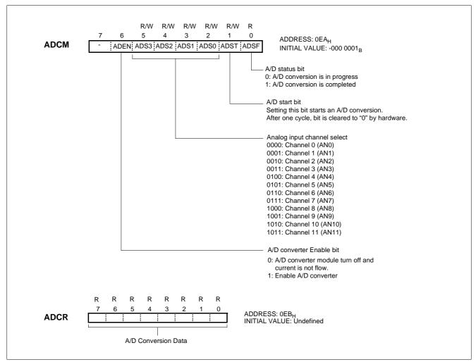
Figure 13-1 A/D Converter Control Register
