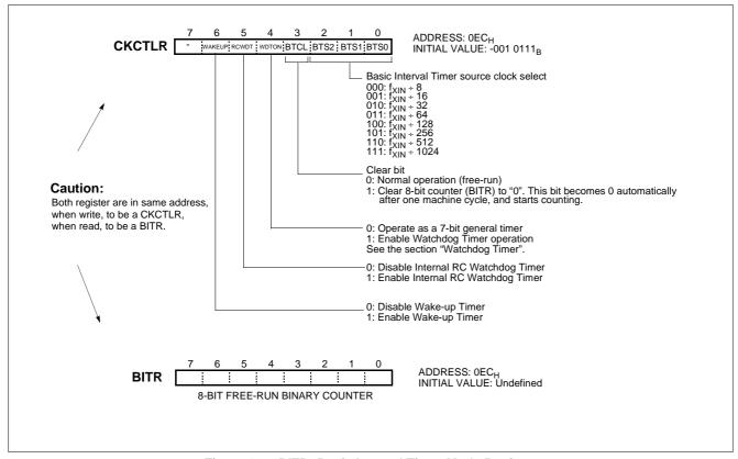
Figure 10-2 BITR: Basic Interval Timer Mode Register
