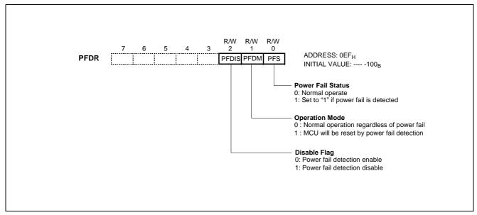
Figure 20-1 Power Fail Voltage Detector Register
