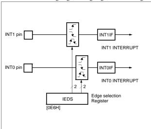
Figure 16-7 External Interrupt Block Diagram
