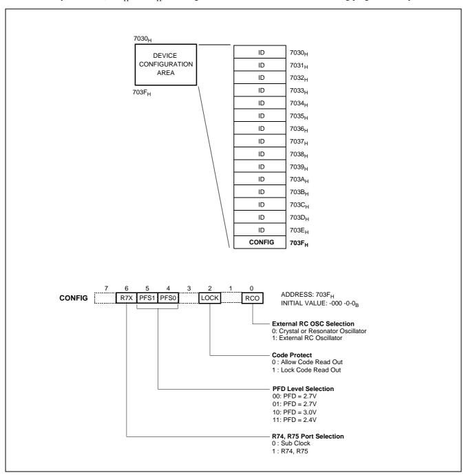
Figure 21-1 Device Configuration Area
