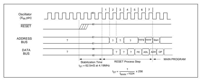
Figure 19-2 Timing Diagram after RESET
