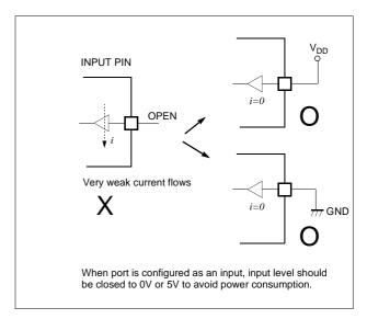
Figure 17-7 Application Example of Unused Input Port
