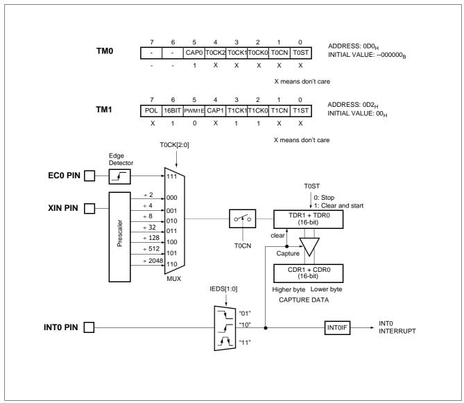
Figure 12-11 16-bit Capture Mode
