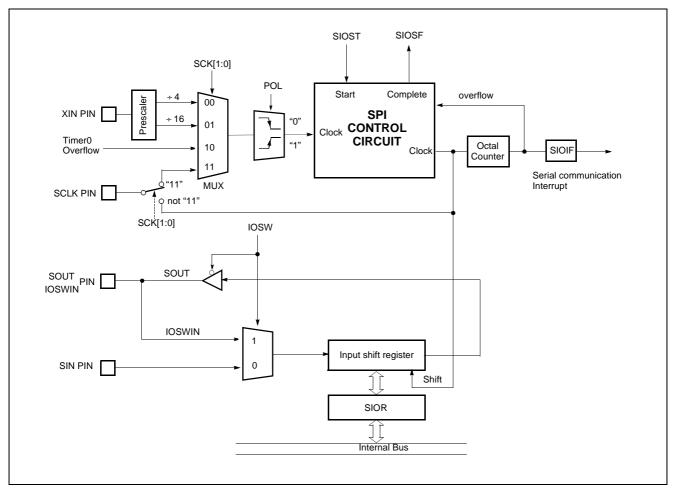
Figure 14-1 SPI Block Diagram
