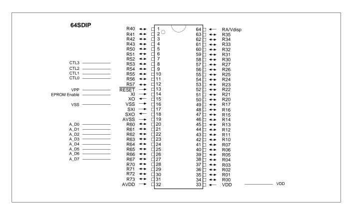
Figure 21-2 Pin Assignment (64SDIP)
