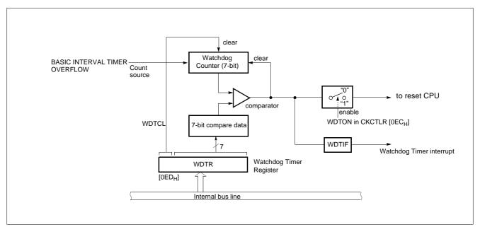
Figure 11-1 Block Diagram of Watchdog Timer
