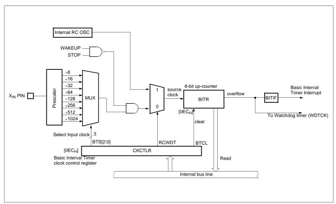
Figure 10-1 Block Diagram of Basic Interval Timer
