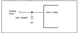
Figure 13-4 Analog Input Pin Connecting Capacitor
