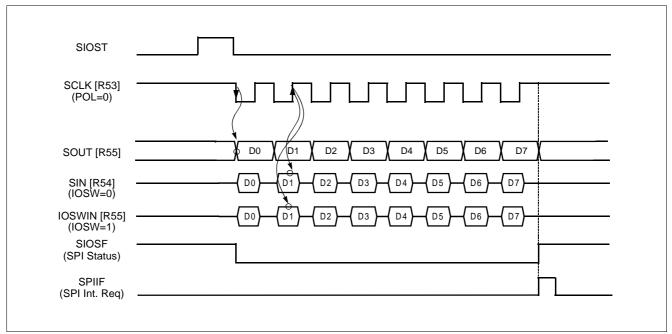
Figure 14-3 SPI Timing Diagram at POL=0
