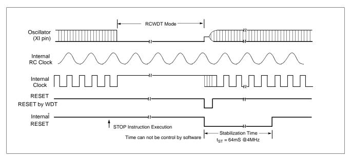
Figure 17-6 Internal RCWDT Mode Releasing by RESET
