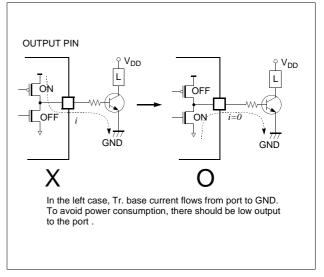
Figure 17-8 Application Example of Unused Output Port
