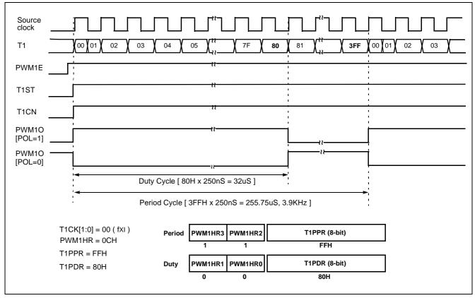
Figure 12-13 Example of PWM at 4MHz
