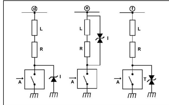
$V_{CL}$  is the voltage (measured) at the terminals of the Transil when the load current goes through it.
