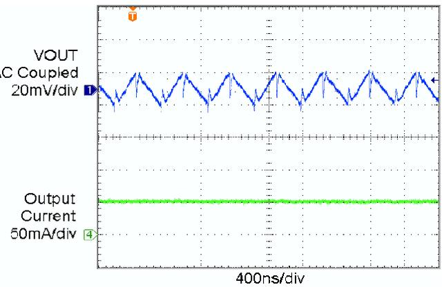
Figure 19. Output Ripple Voltage ( $I_{OUT} = 50\text{ mA}$ )
