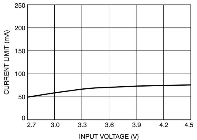
Figure 7. Short Circuit Current vs. Input Voltage
