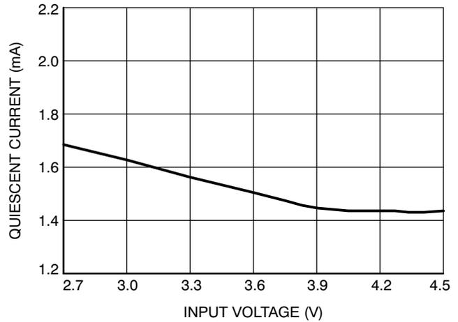
Figure 3. Quiescent Current vs. Input Voltage (No Load)
