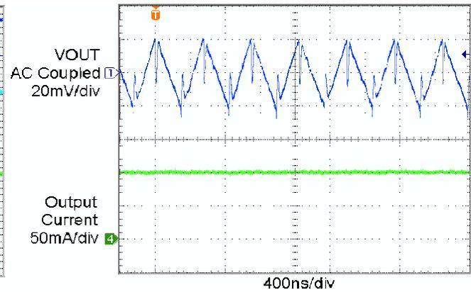
Figure 11. Output Ripple Voltage ( $I_{OUT} = 100\text{ mA}$ )
