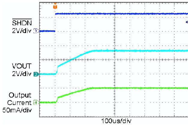
Figure 18. Power Up Waveform ( $I_{OUT} = 50\text{ mA}$ )
