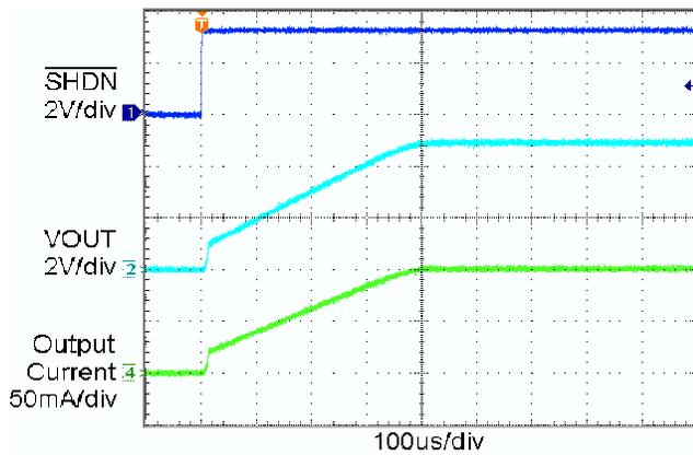
Figure 10. Power Up Waveform ( $I_{OUT} = 100\text{ mA}$ )
