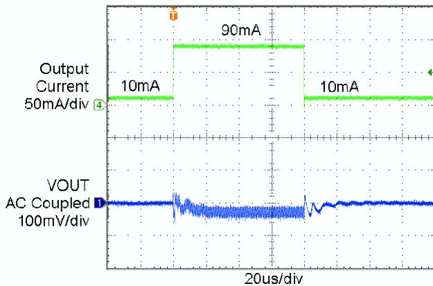
Figure 12. Load Transient Response
