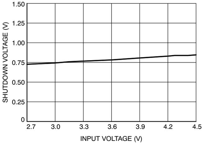
Figure 2. Shutdown Input Threshold vs. Input Voltage
