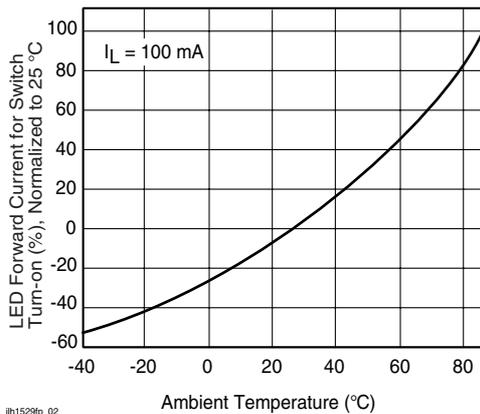
Figure 2. LED Current for Switch Turn-on vs. Temperature
