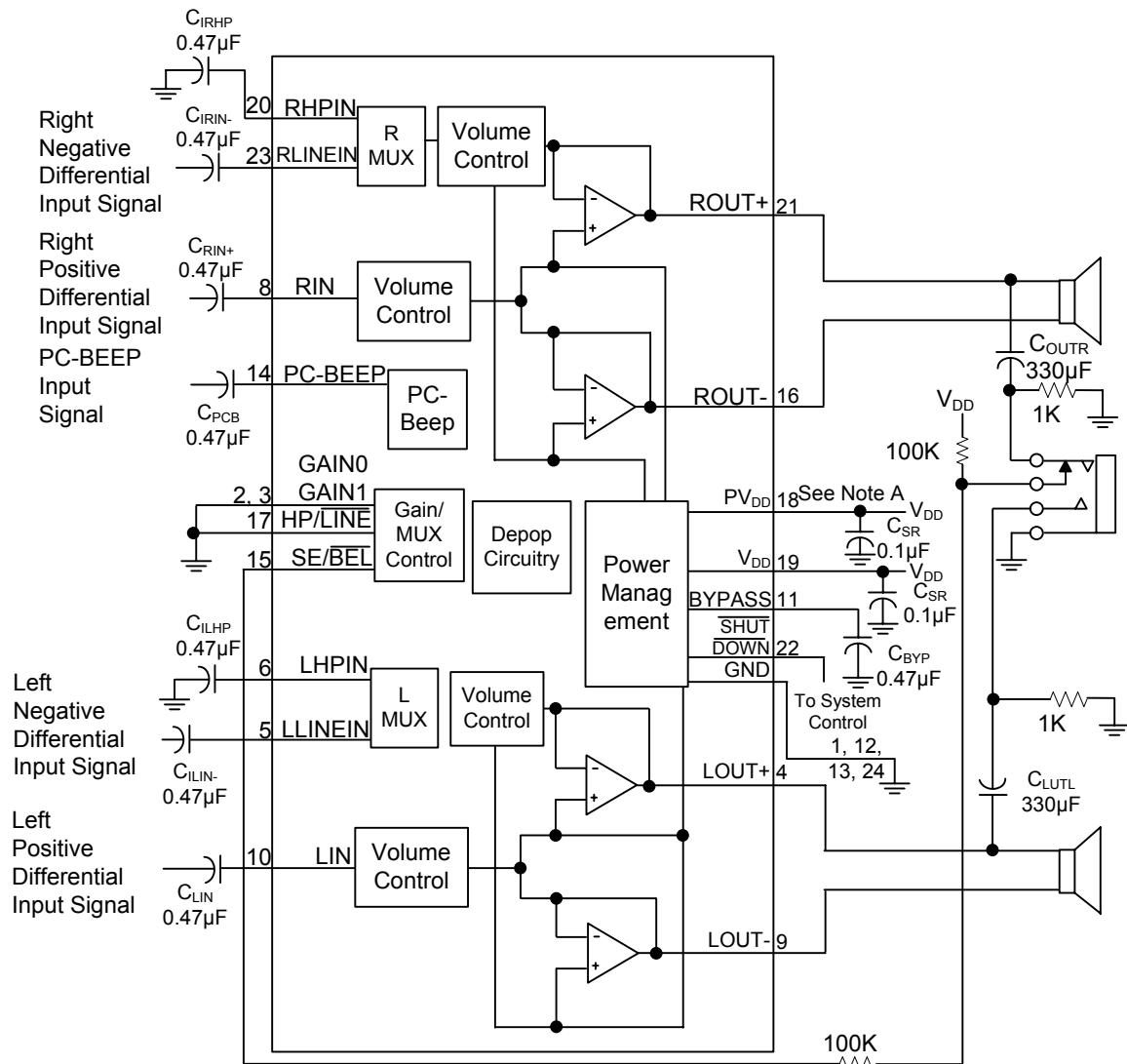
A. A 0.1- $\mu$ F ceramic capacitor should be placed as close as possible to the IC. For filtering lower frequency noise signals, a larger electrolytic capacitor of 10  $\mu$ F or greater should be placed near the audio power amplifier.
