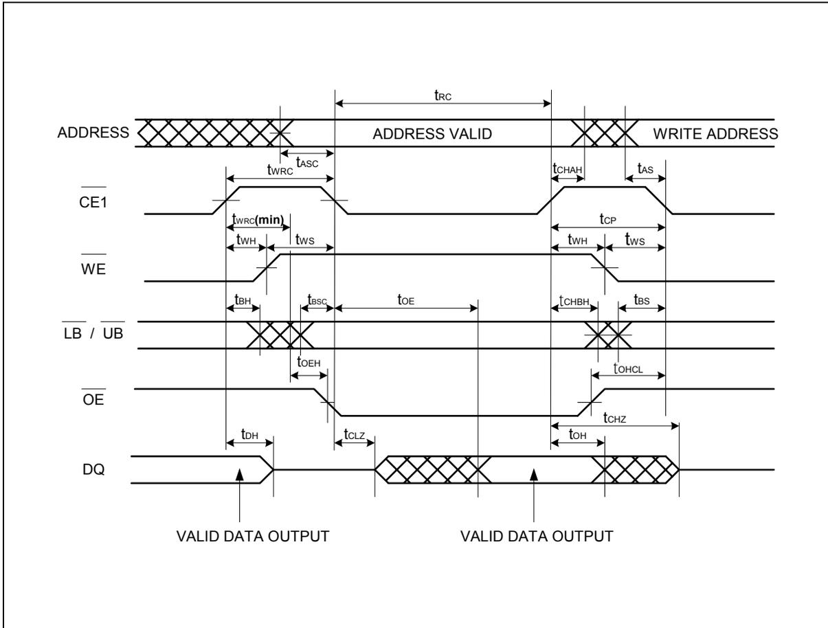
**Note:** The  $t_{OE}$  is specified from the time satisfied both  $t_{WRC}$  and  $t_{WRC(min)}$ .
