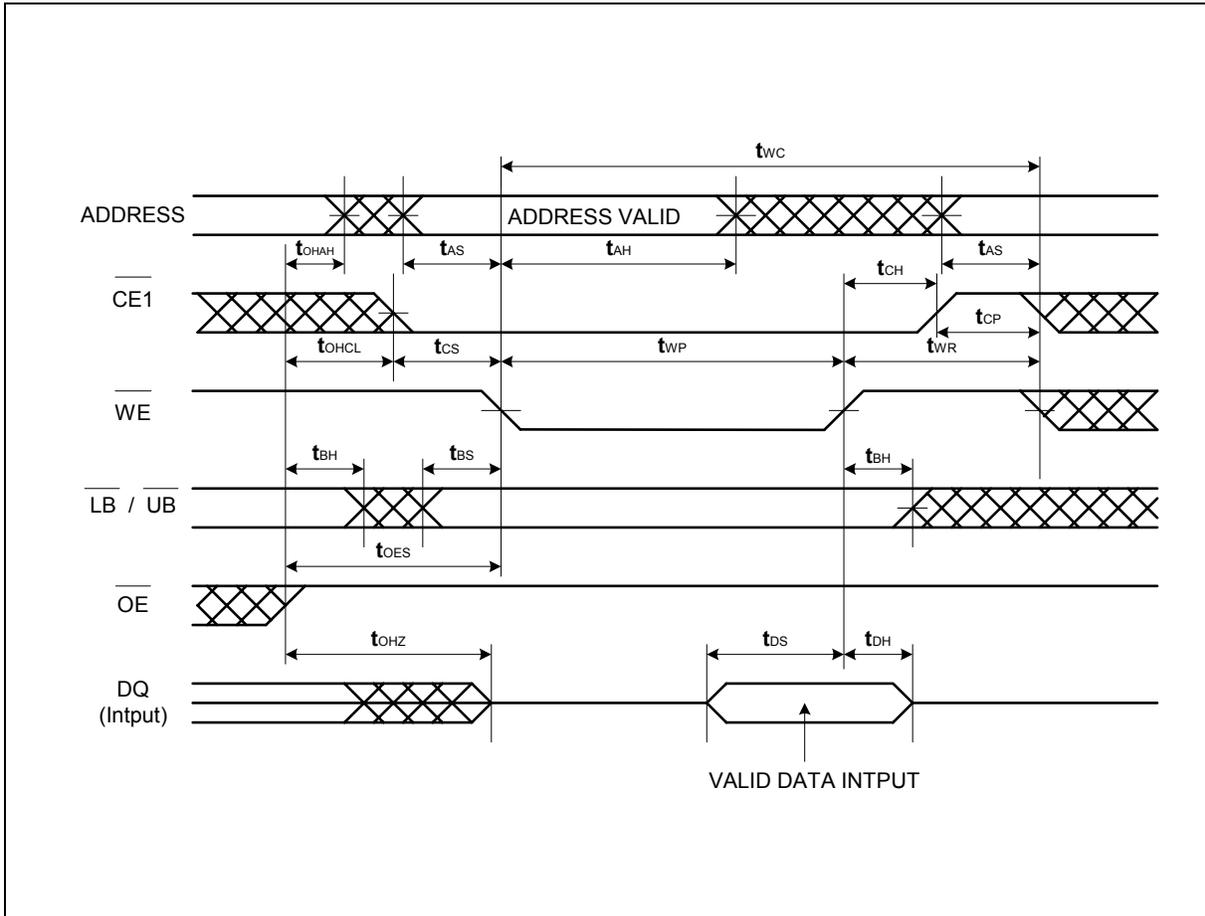
**Note:** CE2, and  $\overline{\text{PE}}$  must be High for entire write cycle.
