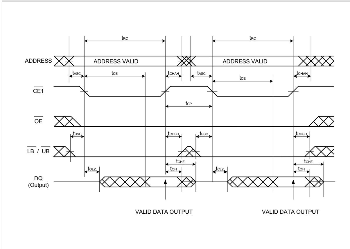
**Note:**  $\overline{\text{CE2}}$ ,  $\overline{\text{PE}}$  and  $\overline{\text{WE}}$  must be High for entire read cycle.
