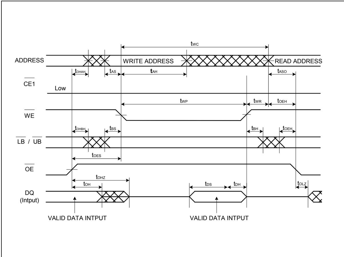
**Note:**  $\overline{CE1}$  can be tied to Low for  $\overline{WE}$  and  $\overline{OE}$  controlled operation.
