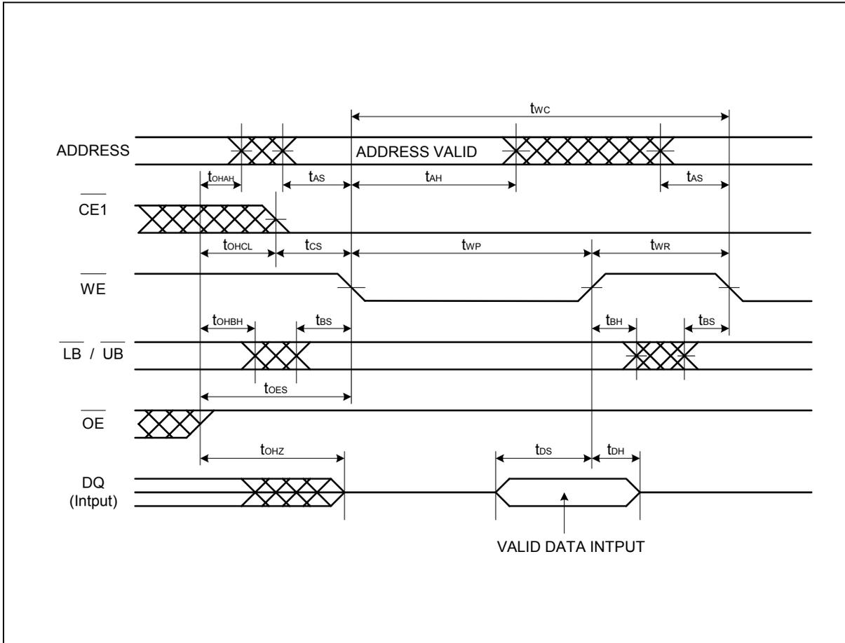
**Note:** CE2 and PE must be High for entire write cycle.
