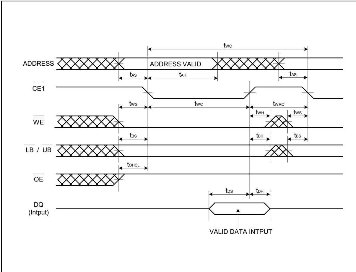
**Note:**  $\overline{\text{CE2}}$ , and  $\overline{\text{PE}}$  must be High for entire write cycle.
