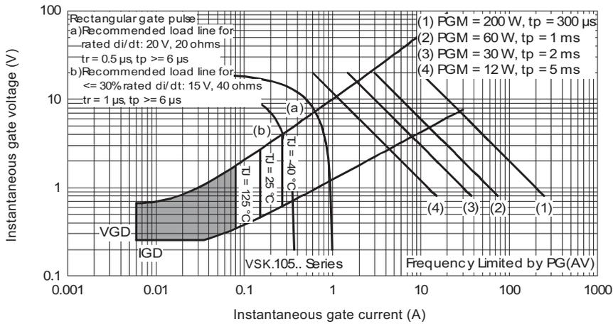
Fig. 11 - Gate Characteristics
