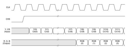
Figure 7. YCbCr to RGB Timing, MODE = 001
