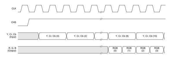
Figure 17. YCbCr to RGB Timing, MODE = 110
