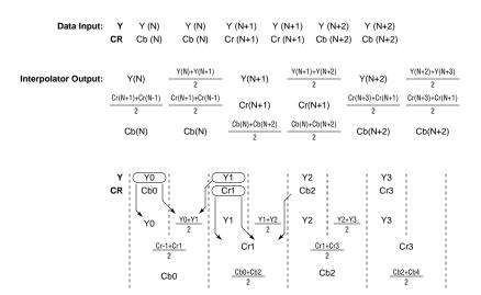
Figure 19. Illustration of Interpolation, MODE = 111
