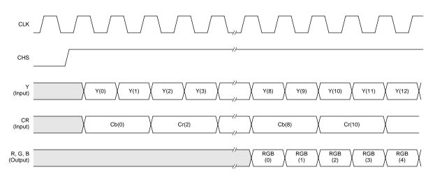
Figure 13. YCbCr to RGB Timing, MODE = 011
