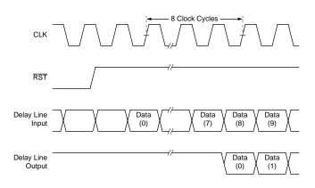
Figure 2. Delay Line Reset Timing
