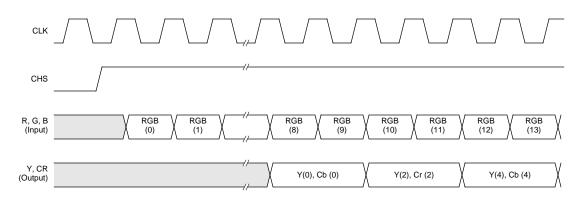
Figure 20. RGB to YCbCr Timing, MODE = 111
