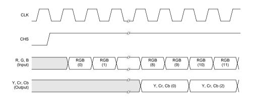
Figure 16. RGB to YCbCr Timing, MODE = 110
