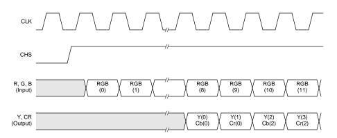
Figure 6. RGB to YCbCr Timing, MODE = 001
