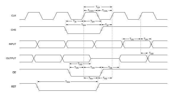
Figure 24. Input Timing Requirements and Output Switching Characteristics
