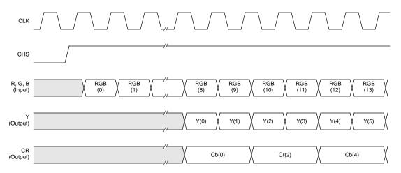
Figure 12. RGB to YCbCr Timing, MODE = 011
