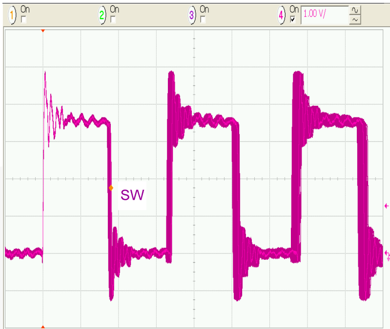
Figure 39. SW-Node Jitter (Infinite Persistence), I_{LOAD} = 200mA , 50ns/div.
