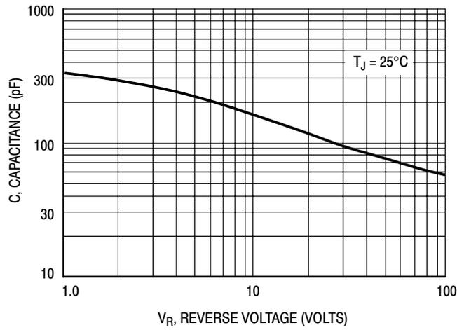
Figure 10. Typical Capacitance
