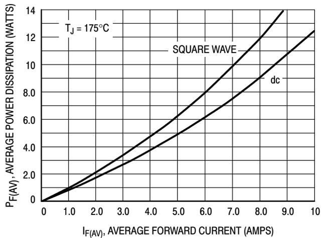
Figure 5. Power Dissipation
