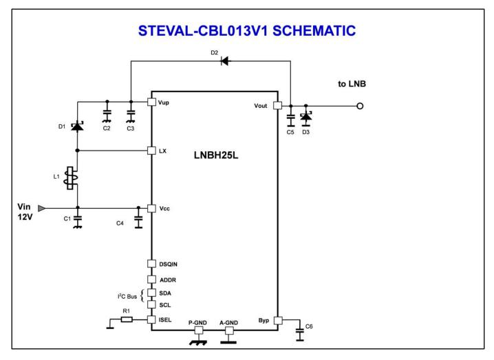
Figure 1: STEVAL-CBL013V1 schematic
