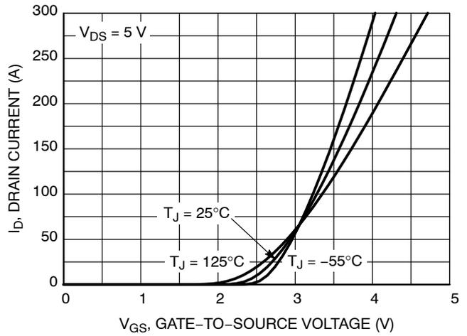
Figure 2. Transfer Characteristics
