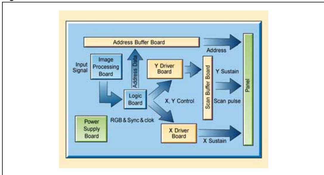
ST's extensive portfolio covers the whole solution for an energy recovery circuit (ERC), sustain circuit, path circuit, and set-reset circuit, both from a power device and IC driver perspective.
