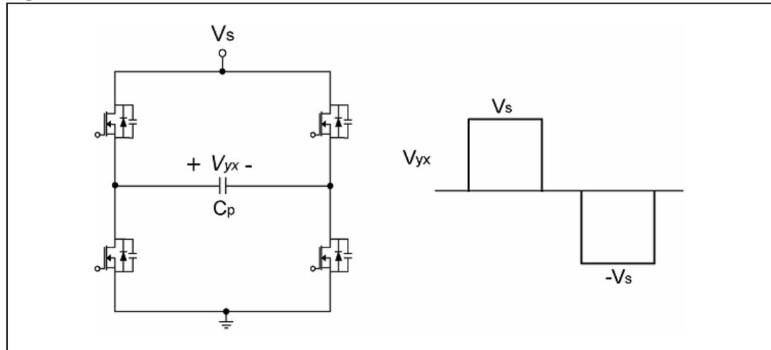
The power dissipation in the sustainer is then  $2C_P V_S^2 f_{av}$ , where  $f_{av}$  is the average sustain cycle frequency.
