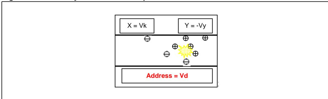
Charges, called wall charges (or wall voltage  $V_w$ ), deposit on the dielectric layer and reduce the effective voltage across the gap. Then, the discharge ceases after a short time, as shown in [Figure 5](#).
