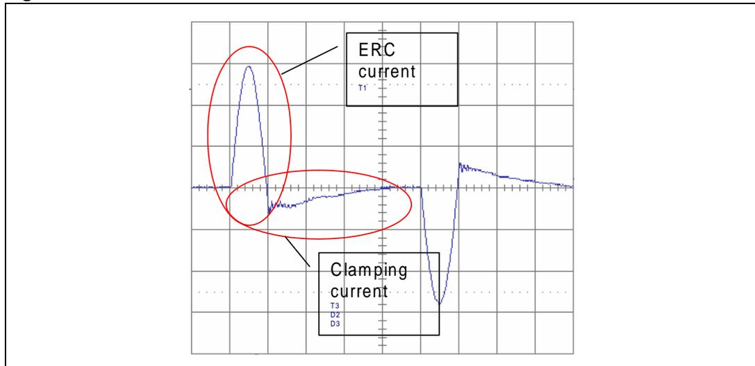
For ER circuit new devices with low voltage drop and very fast turn ON have been developed.
