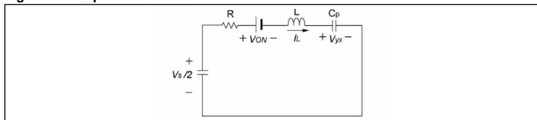
In [Figure 14](#), R represents the parasitic resistance including on-resistances of switches and  $V_{ON}$  represents the diode forward drop. Based on this figure, the panel voltage  $V_{yx}$  can be obtained as follows:
