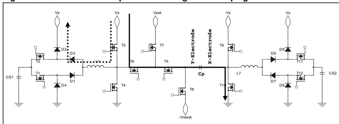
**Figure 17. Circuit scheme – clamping to ground**
