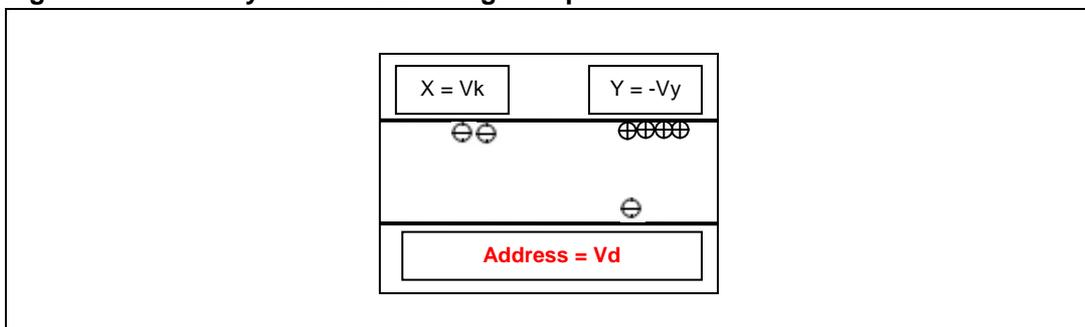
When the polarity of the sustain pulse is reversed, the potential difference across the gap becomes larger than  $V_{bd}$  by an amount determined by the wall charges, and a new large discharge of different polarity occurs, as shown in [Figure 6](#).
