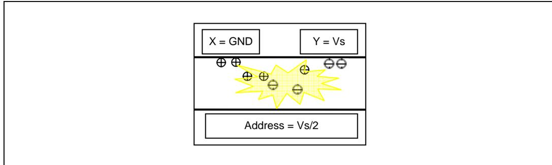
The build-up of wall charges again terminates the discharge, as shown in [Figure 7](#).
