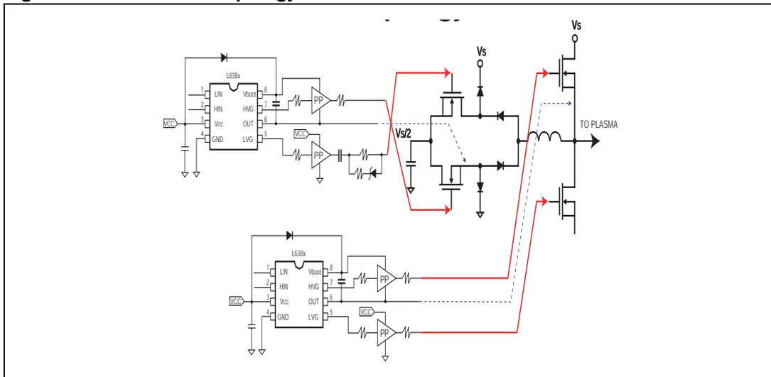
Due to current value in bootstrap charge, the internal diode cannot be used, thus external diode SMBY01-400 [20.] must be used. Further details on L6585 and L6588 application can be found in [18.] and [19].
