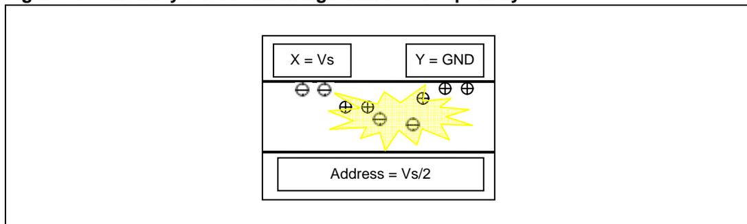
Once the discharge is initiated, it continues as long as the sustain pulse is applied. Due to this memory characteristic of AC PDPs, lower sustain voltage ( $< V_{bd}$ ) pulses can maintain the ac PDPs to light.
