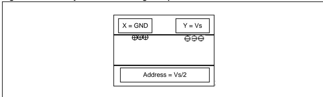
The next discharge starts as the polarity of the sustain pulse is reversed, as shown in [Figure 8](#).
