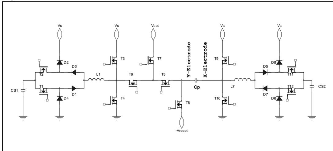
Weber topology provides a new sustainer circuit that recovers the energy otherwise lost in charging and discharging the panel capacitance,  $C_p$ . The efficiency with which the sustainer recovers this energy is defined as the "recovery" efficiency. In particular, when  $C_p$  is charged to  $V_s$  and then discharged to zero, the energy that flows into and out of  $C_p$  is  $E = C_p V_s^2$ .
