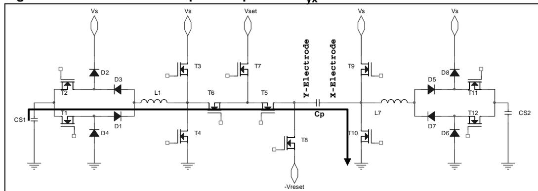
The equivalent circuit during the LC resonant period of the energy recovery circuit is:
