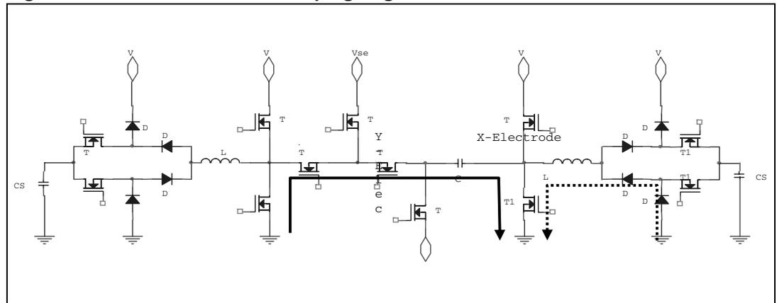
It can be noted that during sustain phase, path switches T5 and T6 are always turned ON, and they see both energy recovery current and discharge current which explains the need for low voltage drop devices.
