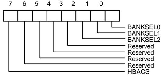
Bit 7: HBACS- High byte access. Set to 1(default), access Register 4Fh high byte register. Set to 0, access Register 4Fh low byte register.
