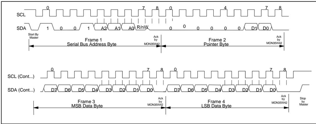
**FIGURE 9 - TEMPERATURE 2/3  $T_{OS}$  AND  $T_{HYST}$  WRITE**
