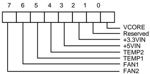
Bit 7-0: A one disables the corresponding interrupt status bit for nSMI interrupt.
