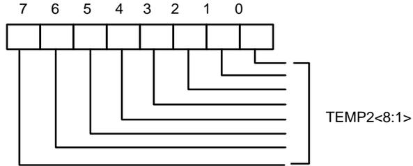
Bit 7-0: Temperature <8:1> of sensor 2, Bit 7 is MSB.
