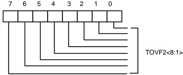
Bit 7-0: Over-temperature bit 8-1, Bit 7 is MSB. The temperature default 80 degree C.
