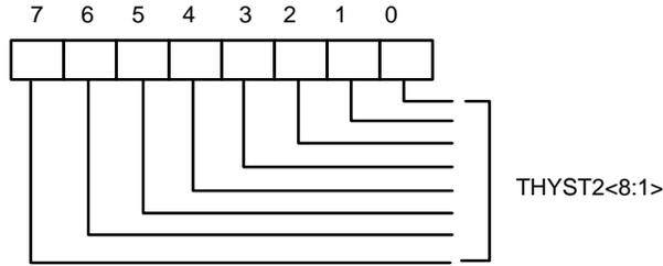
Bit 7-0: Temperature hysteresis bit 8-1, Bit 7 is MSB. The temperature default is 75 degree C.
