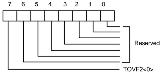
Bit 7: Read/Write - Over-temperature bit 0, LSB.
