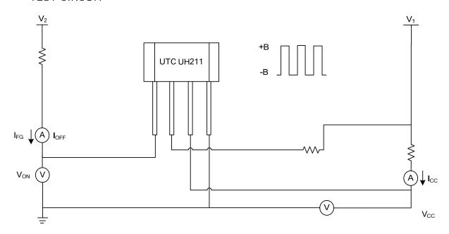
$\label{eq:local_control} \text{Measure V}_{\text{CC}}, I_{\text{CC}} \text{ when DO is off.} \quad \text{Measure V}_{\text{ON}}, I_{\text{FG}} \text{ when FG is on.} \quad \text{Measure I}_{\text{OFF}} \text{ when FG is off.}$
