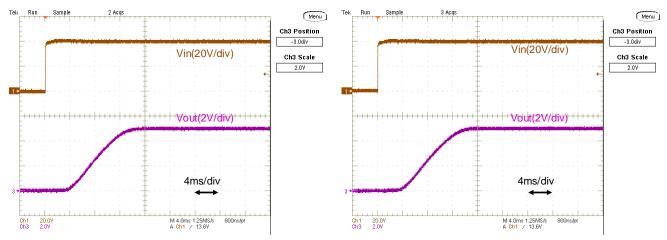
Fig.12-2-13. Start-up Waveform (Io=0A)
