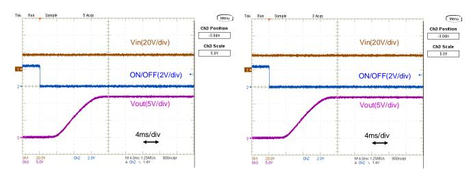
Fig.12-2-21. Start-up Waveform (Io=0A)
