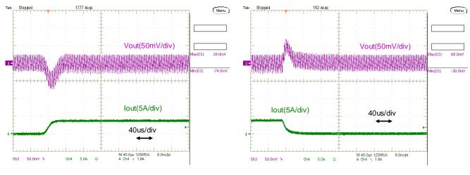
Fig.12-2-11. Load Transient Response (Io=  $0 \rightarrow 3.5A$ )
