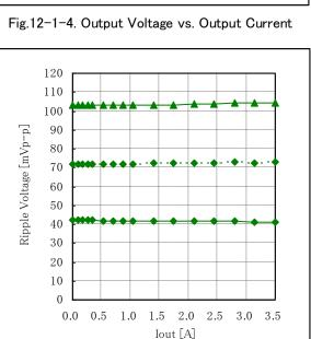
Fig.12-1-6. Ripple Voltage vs. Output Current
