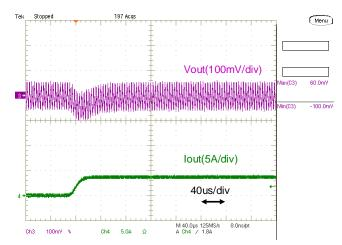
Fig.12-2-35. Load Transient Response (Io=  $0 \rightarrow 3.5A$ )
