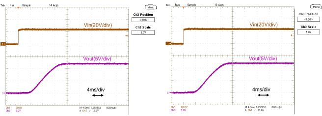
Fig.12-2-25. Start-up Waveform (Io=0A)
