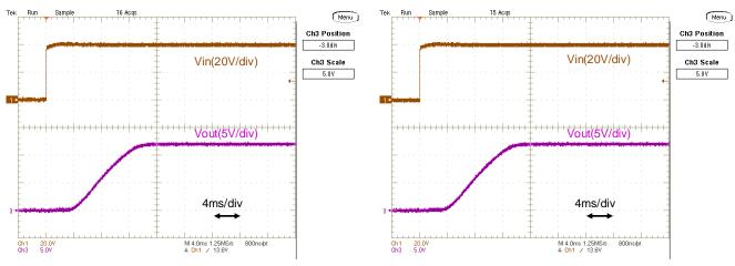
Fig.12-2-31. Start-up Waveform (Io=0A)
