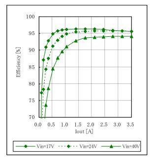
Fig.12-1-5. Efficiency vs. Output Current
