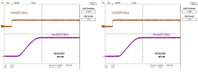
Fig.12-2-1. Start-up Waveform (Io=0A)
