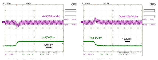
Fig.12-2-29. Load Transient Response (Io=  $0 \rightarrow 3.5A$ )
