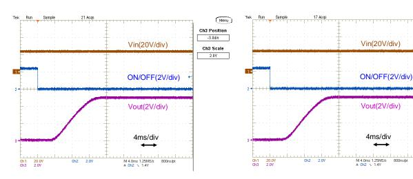
Fig.12-2-9. Start-up Waveform (Io=0A)
