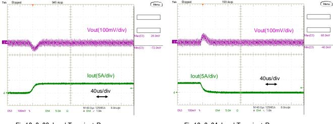
Fig.12-2-23. Load Transient Response (Io=  $0 \rightarrow 3.5A$ )
