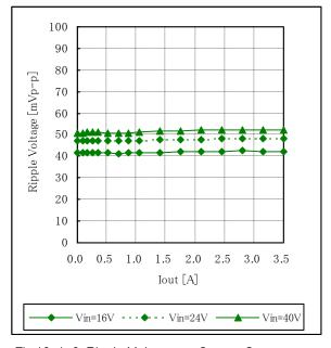
Fig.12-1-3. Ripple Voltage vs. Output Current
