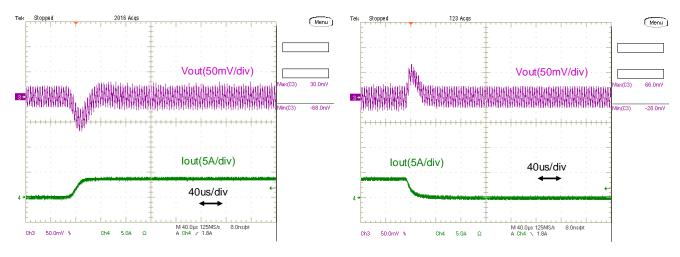
Fig.12-2-5. Load Transient Response (Io=  $0 \rightarrow 3.5A$ )
