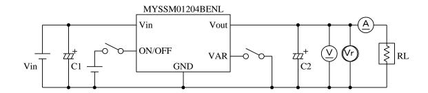
C1: Conductive Polymer Aluminum Solid Electrolytic Capacitor 100µF/50V
