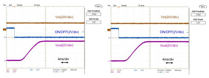
Fig.12-2-3. Start-up Waveform (Io=0A)
