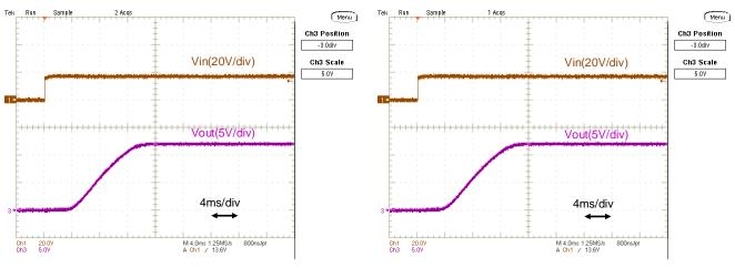
Fig.12-2-19. Start-up Waveform (Io=0A)
