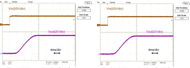
Fig.12-2-7. Start-up Waveform (Io=0A)
