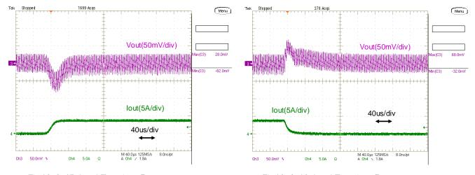
Fig.12-2-17. Load Transient Response (Io=  $0 \rightarrow 3.5A$ )
