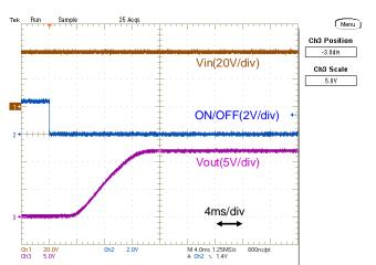
Fig.12-2-33. Start-up Waveform (Io=0A)
