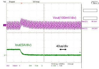
Fig.12-2-36. Load Transient Response (Io=  $3.5A \rightarrow 0$ )
