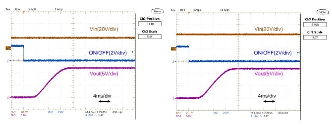
Fig.12-2-27. Start-up Waveform (Io=0A)
