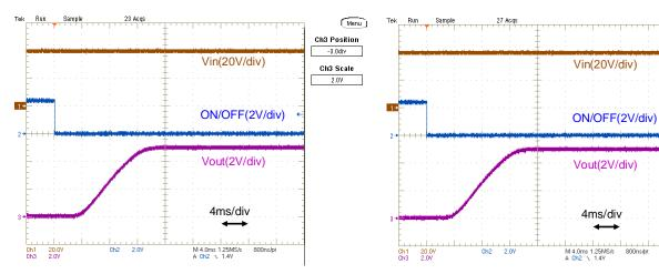
Fig.12-2-15. Start-up Waveform (Io=0A)
