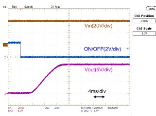
Fig.12-2-34. Start-up Waveform (Io=3.5A)
