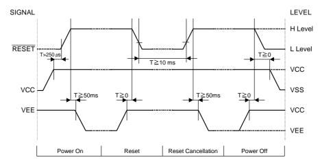
Please maintain the above sequence when turning on and off the power supply of the module. If  $V_{EE}$  is supplied to the module while internal alternate signal for LCD driving (M) is unstable or  $\overline{RESET}$  is active, DC component will be supplied to the LCD panel. This may cause damage to the LCD module.
